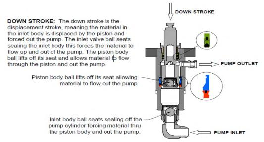
Figure 2. Pump Down Stroke Diagram
