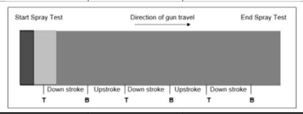
Material delivered at the beginning of the test spray is cold (low catalyst), followed by material that is properly mixed and cures (see below). This indicates that the system is unbalanced at the beginning of the spray.
